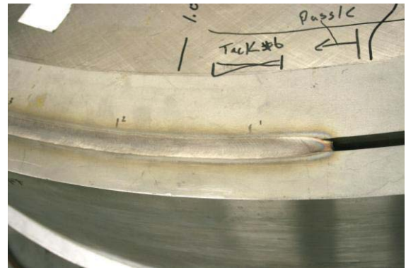
Figure 6. A thick section narrow groove weld in a 316 stainless steel coupon.
